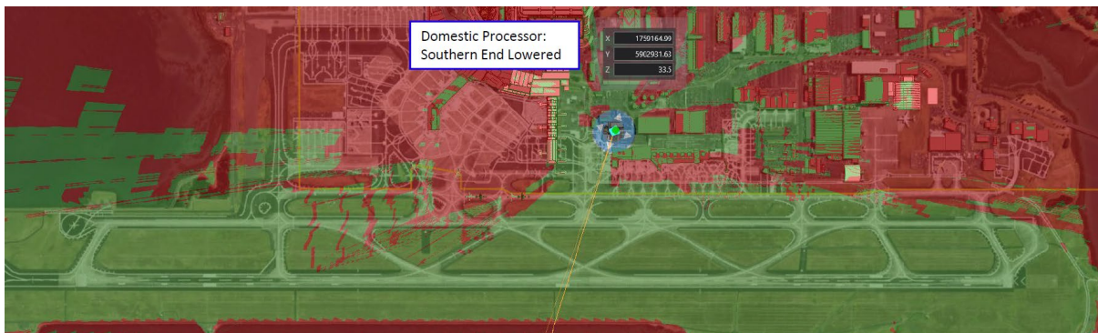
Figure 3 - Visibility from current ATC Tower post Pier A1 Construction
